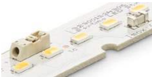
Example of a fuse mounted on a LED module
